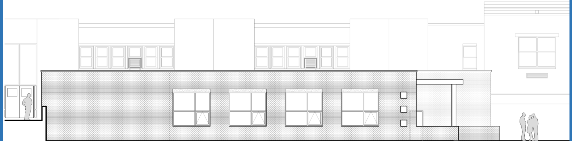
2 PROPOSED EAST ELEVATION AT CAFETERIA SCALE: 1/4" = 1'-0"
